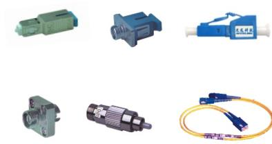
Optical fixed attenuator include ordinary fiber gap based adaptor-like attenuator (OAT-F),attenuation fiber based attenuator with low back reflection (OAT-HF), and in-line structure attenuator(OAT-HFI).The attenuators could be selected with different connector types.
